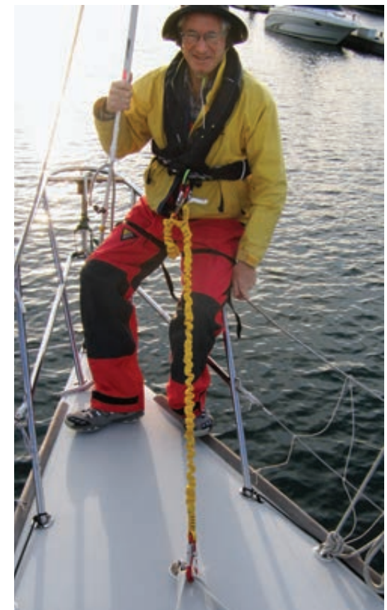
The jacklines end short of the bow and stern to help prevent falls and keep people on deck when they happen.
